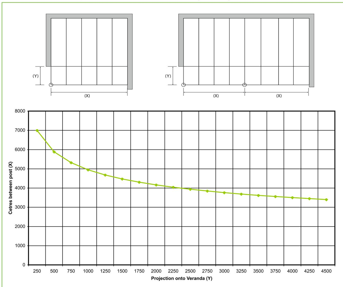
For loading condition other than 0.6kn/m2 (with 4-16-4 glass units) please let our specification team know. Ultraframe's U-Design software simply needs your home postcode to calculate the loads and the resulting roof specification.
